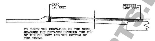
Under normal tension, the neck should have a slightly concave curvature. Creating a counteracting force, the truss rod prevents the neck from bending excessively under the stress placed on it by the strings. The tension on the rod is adjustable so the correct curvature can be achieved by regulating the neck's resistance to string tension.
